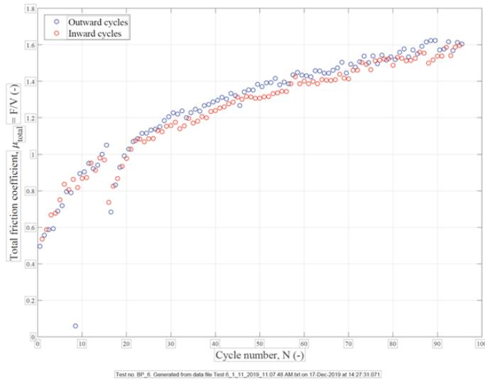
Increase in soil resistance with cyclic soil consolidation.
