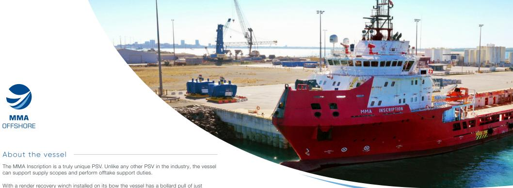
With a render recovery winch installed on its bow the vessel has a bollard pull of just over 65 tonnes. MMA undertook the bespoke modification in 2015 after we identified an opportunity to innovate our client's marine activities in the Timor Sea.
